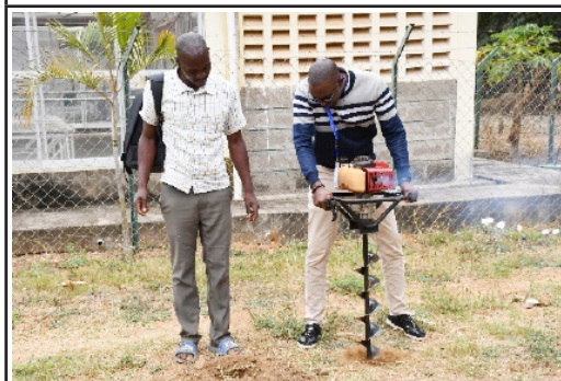
Figure 4.24: Demonstration of soil auger for planting long-rooted seedlings
