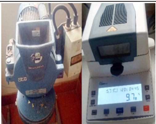
Figure 4.11: Grinder and moisture meter to test the moisture content of seeds
